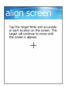
• Press the stylus to the targeted center target accurately, and doing the same when the target move to up left, down left, down right, up right (This is to settle the input value of stylus in LCD screen.
